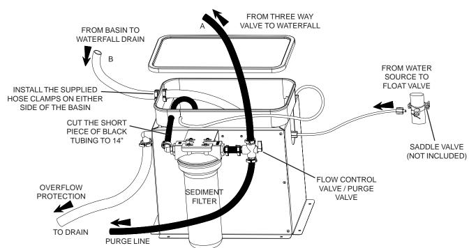
Remove components from basin and assemble as shown. The fittings required are already attached to the filter and basin. Measure and cut the lines to the length necessary, push onto the barbed fittings and secure with the supplied hose clamps. Leak test the waterfall before fully enclosing.
